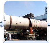
Raw meal is heated at a temperature of ~1,450 °C in a cement kiln to produce clinker.
